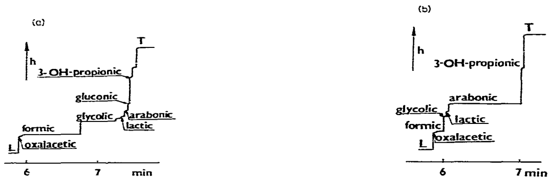
Fig. 1. Mother-liquor after potassium arabonate crystallization. Sample injected: 1 \mu l of sample diluted 1:100. (b) Potassium arabonate crystalloid. Sample injected: 5 \mu l of 0.2% solution. h = Detector signal. Leading (L) and terminating (T) anions were chloride and propionate, respectively.
